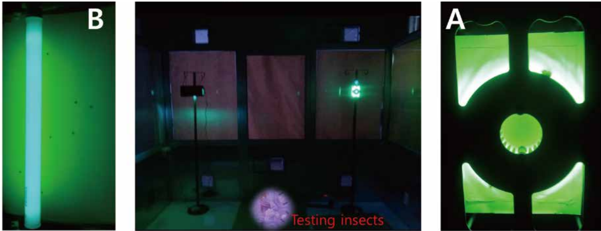
Figure 1: Experiment on Light trap A and B in the 27 m 3 room-size chamber.
