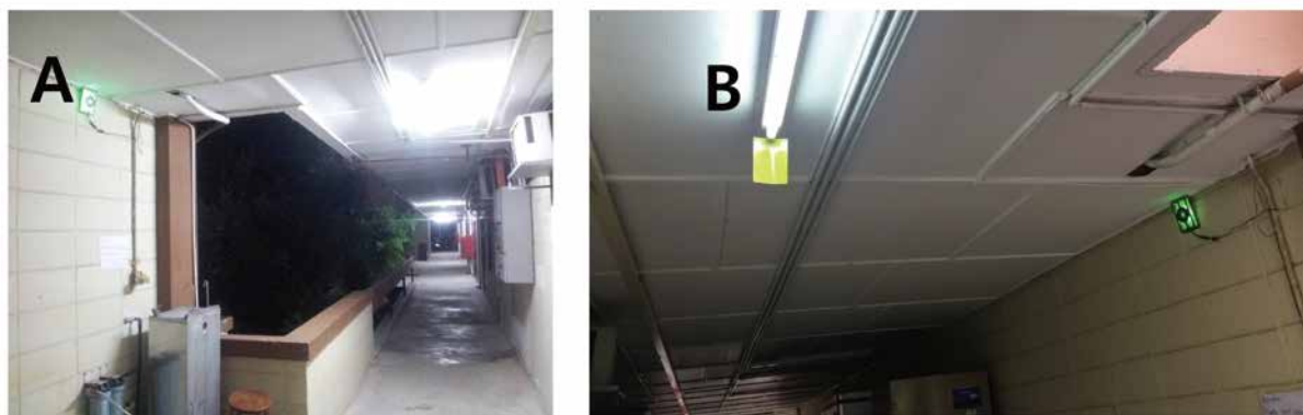
Figure 2: The field evaluation of the insect attractions to Light trap A versus that of the regular fluorescent light.
